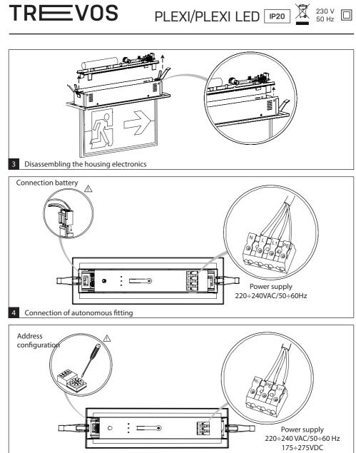
4a Connection and setup of fitting to central battery
